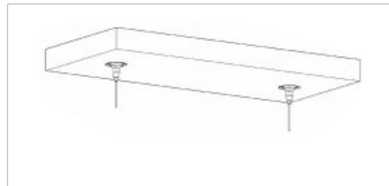
2. Rubber plug and screw is used to fix the clamp on the ceiling
